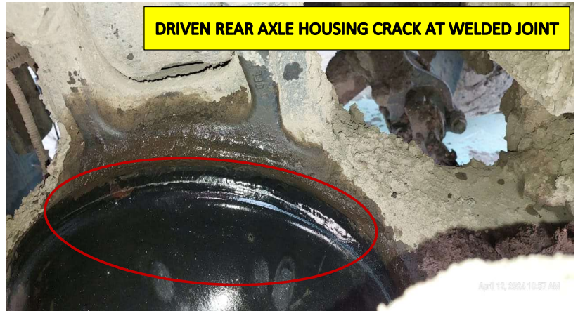
DRIVEN REAR AXLE HOUSING CRACK AT WELDED JOINT
