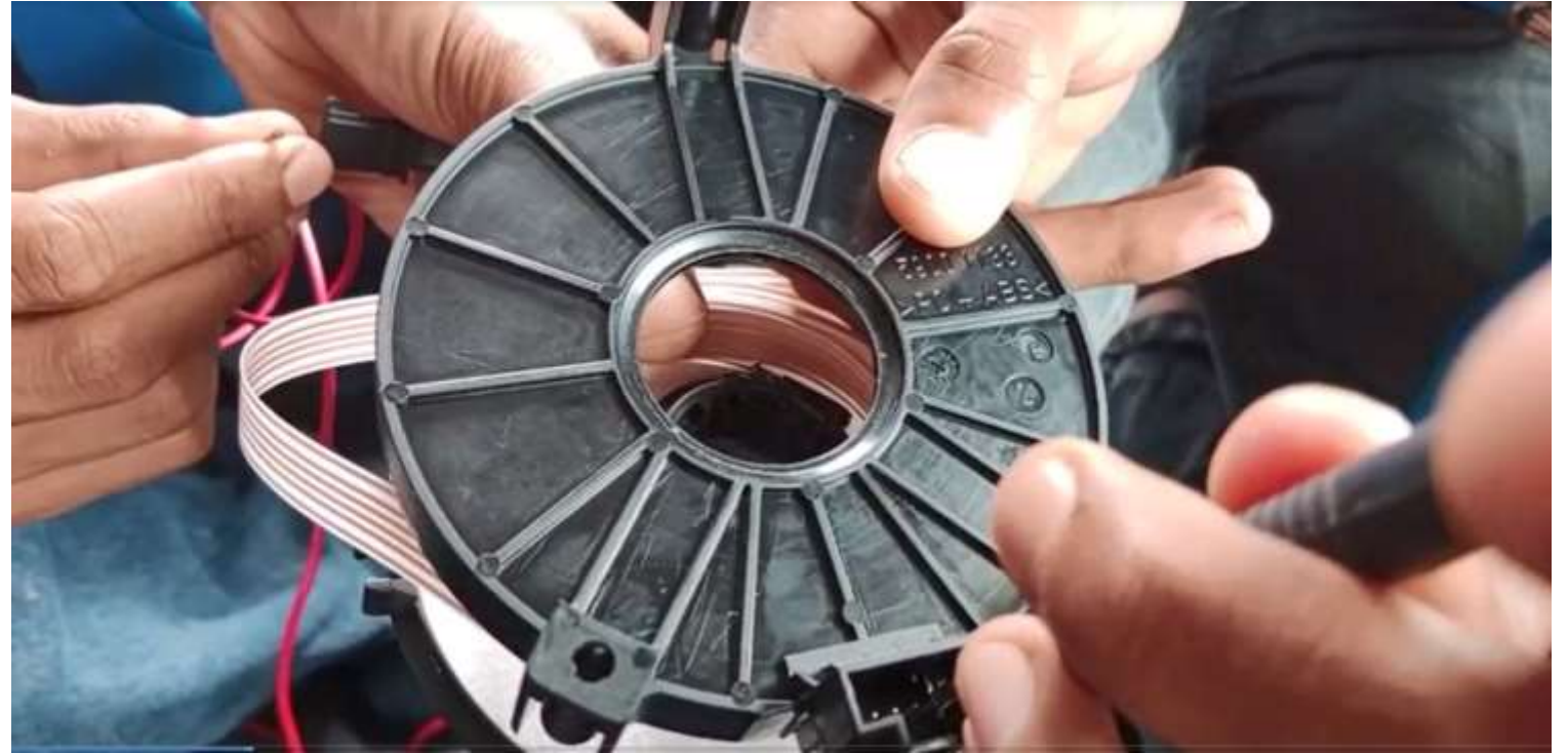
Pengecekan continuitas kabel clock spring steering
