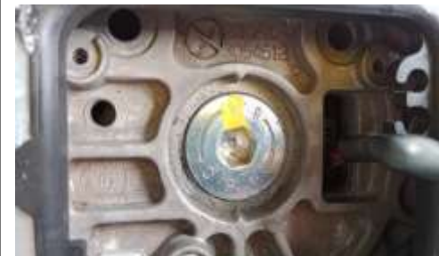
Melepas Bolt steering wheel
