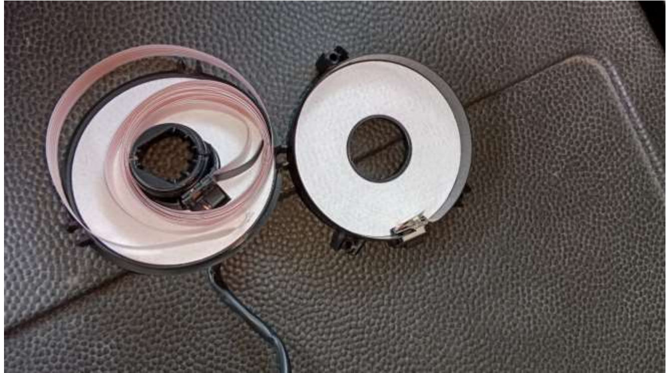
Pengecekan kabel clock spring steering
