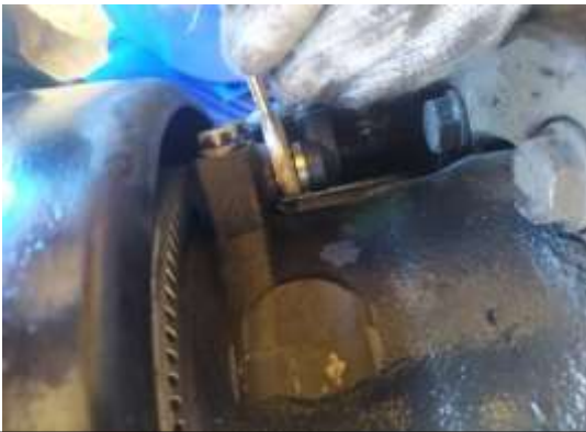
Proses pemasangan sensor wheel speed
