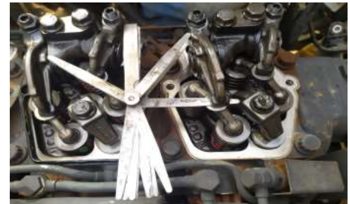
Pengecekan valve clearance
