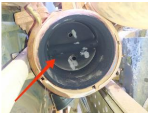
Posisi flap tertutup (normally open)
